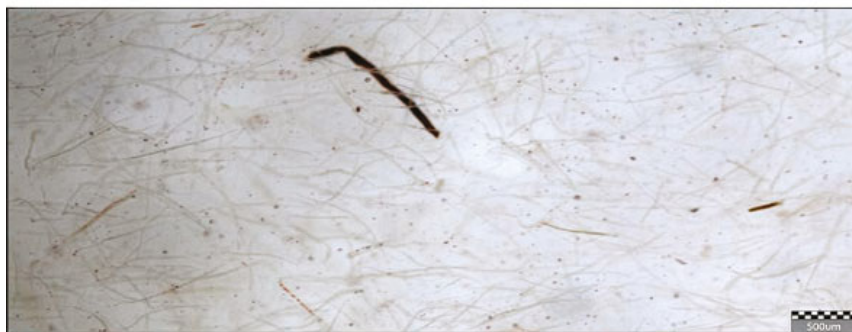
Image 3: BIM Pics image where pitch has been visualised by staining the sample with a dye that binds to pitch. This makes it possible to distinguish internal pitch from external pitch.
