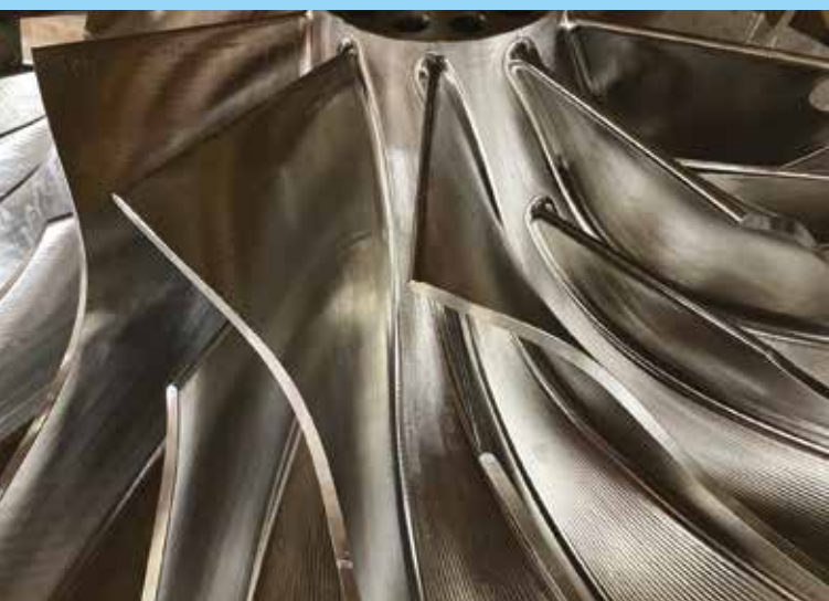
Image 2: Runtech open impeller.tif: The open (shroudless) impeller design was developed to meet two critical needs: lower maintenance requirements and reduced energy consumption per ton..
