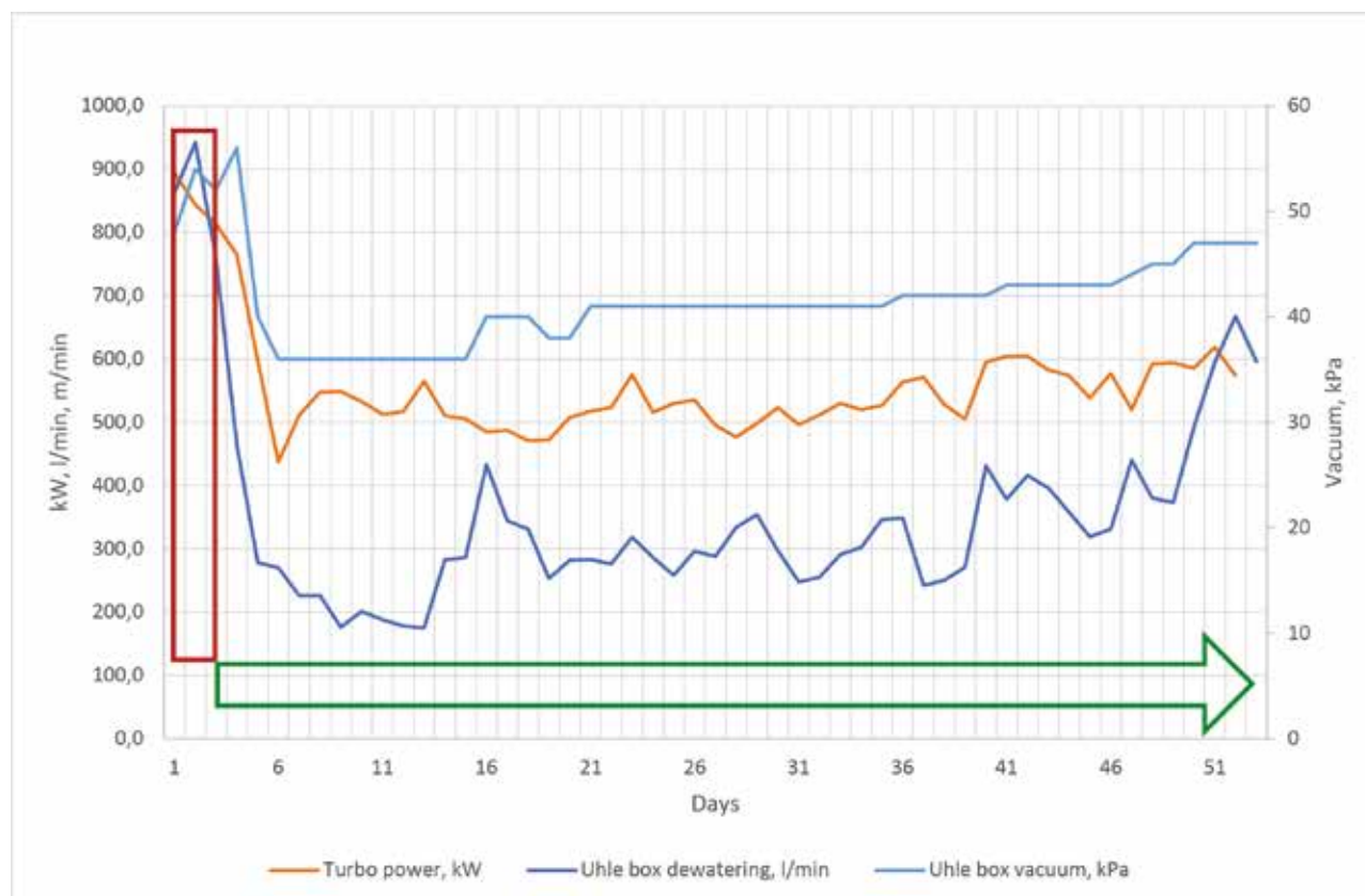
Figure 4: Air flow and energy consumption variance during a felt lifecycle.
