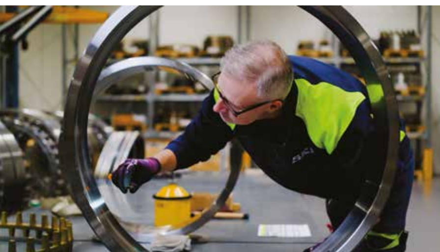
Image 3: (Left) Circular solution centre inspect bearing.
