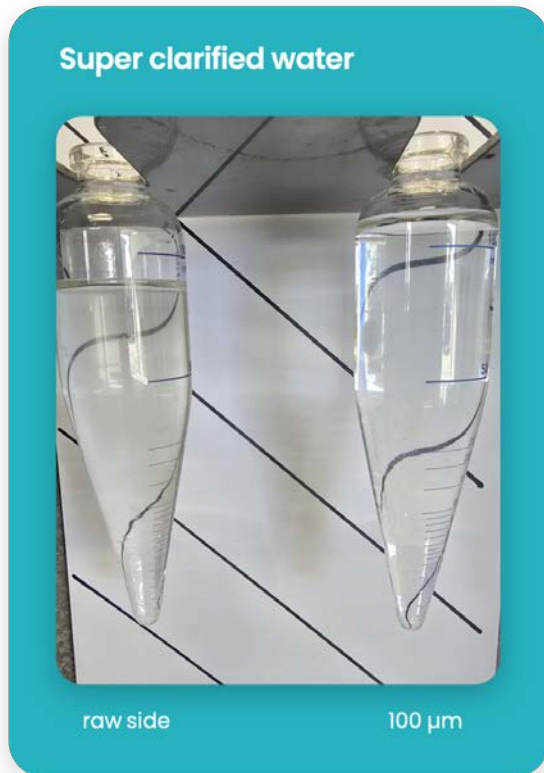
Figure 8: Filtration of the super-clear filtrate from a specialty paper mill. The turbidity caused by fibres was reduced, and all particles larger than 99 µm were removed.
