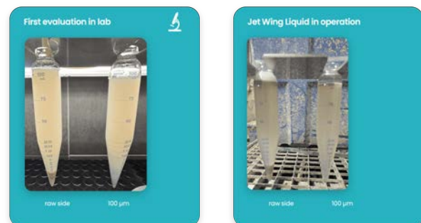
Figure 7: Laboratory test with clear filtrate on the left, and results using the Jet Wing Liquid Filter in normal operation on the right.
