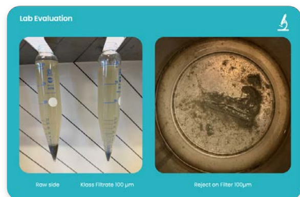
Figure 9: Clarified water and Klass filtrate from a fine paper mill, as well as screen residue.
