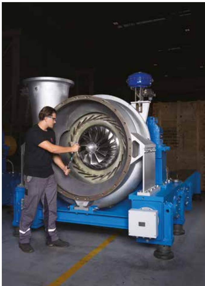
Image 5: The RT-type TURBAIR® vacuum blowers were manufactured at Everllence Switzerland' Zurich factory ©Andrin Winteler / Everllence
