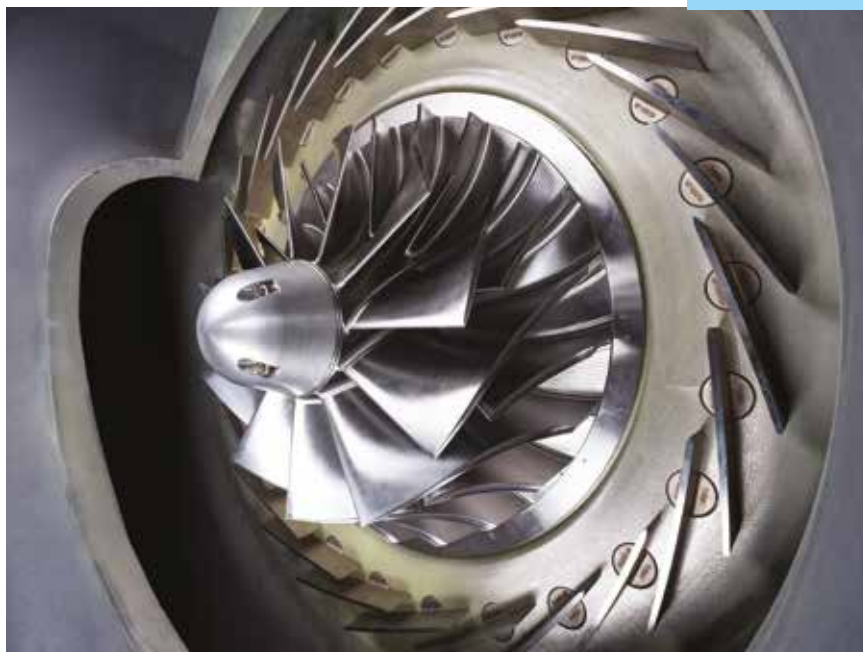
Image 3: TURBAIR® systems use air and high-speed impellers – instead of water – to create vacuum and remove moisture from the paper web. © Andrin Winteler / Everllence
