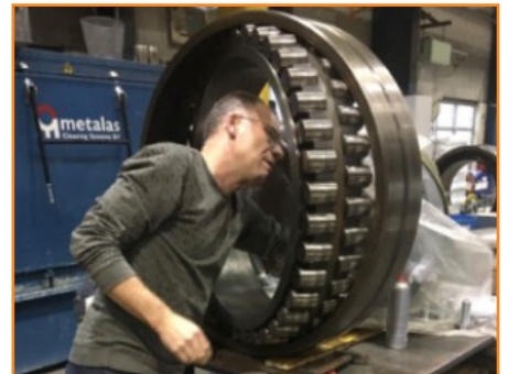
SKF Application Engineer pre-inspecting the bearing on-site
