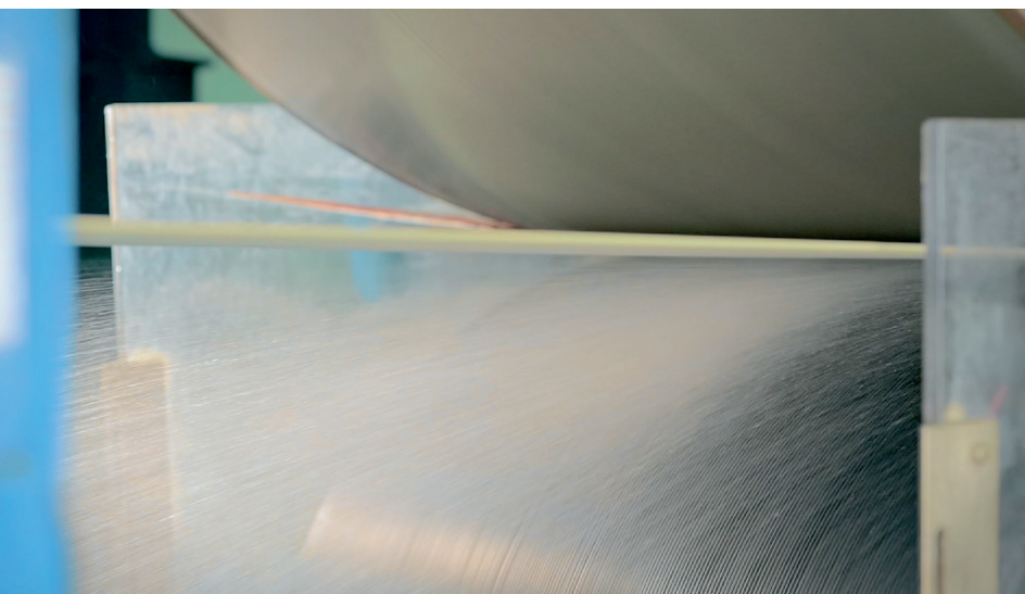
Figure 4a: (Below) Good nip dewatering
