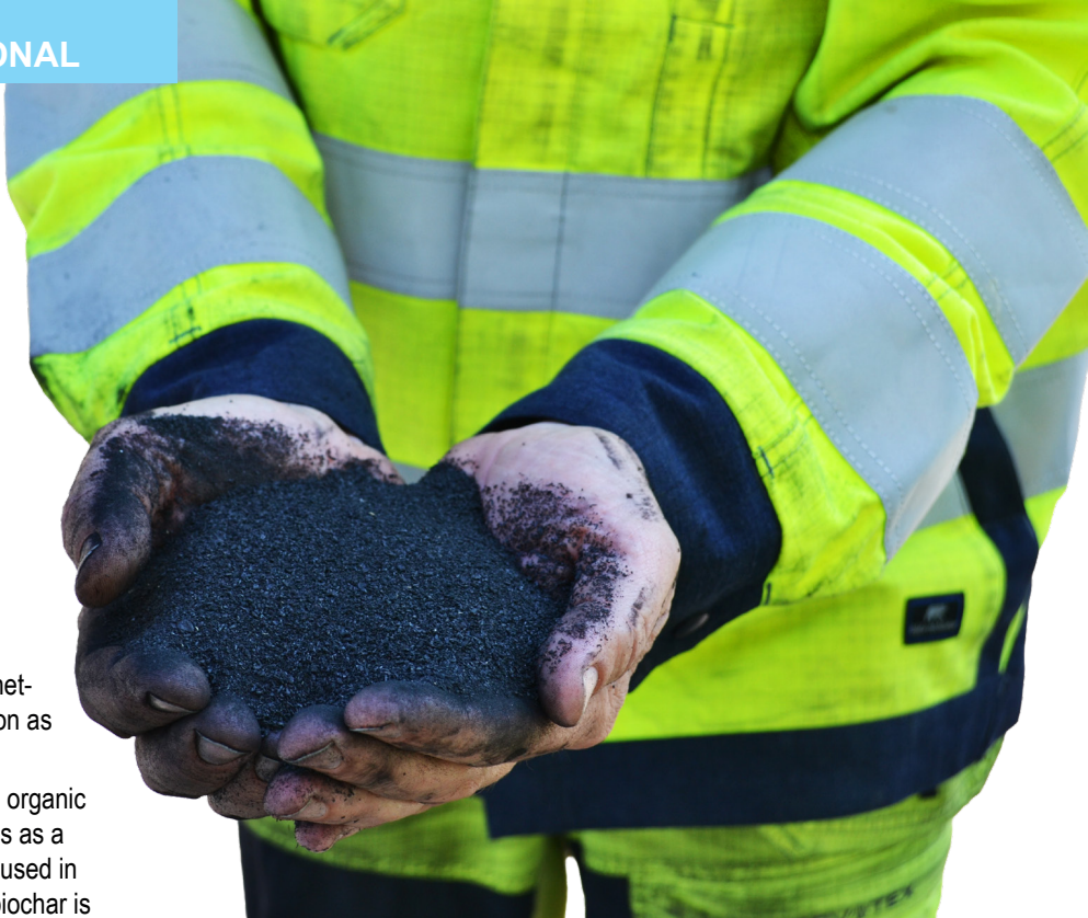
Figure 2: Biochar - a valuable by-product from biomass gasification.
