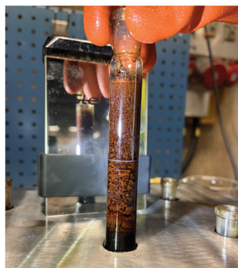
Figure 5a and 5b: Separation of soap from black liquor without dosage of BIM soap booster. 5b: Separation of soap from black liquor with dosage of BIM soap booster. A more compact layer of soap with less black liquor in the soap.
