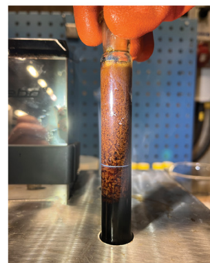
Figure 5a and 5b: Separation of soap from black liquor without dosage of BIM soap booster. 5b: Separation of soap from black liquor with dosage of BIM soap booster. A more compact layer of soap with less black liquor in the soap.
