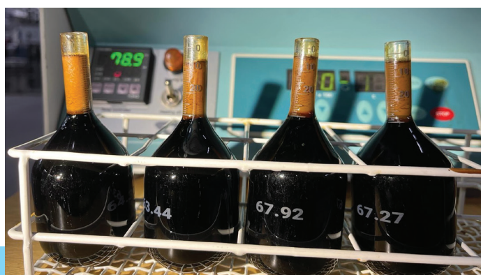
Figure 6: Centrifuge test to analyse separable soap content.
