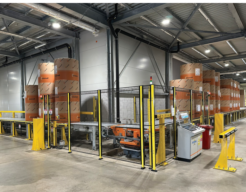
Figure 6 & 7: Up-ended roll stacks sorted on warehouse conveyor right after ARW for one touch "pick – turn - load" shipping process.
