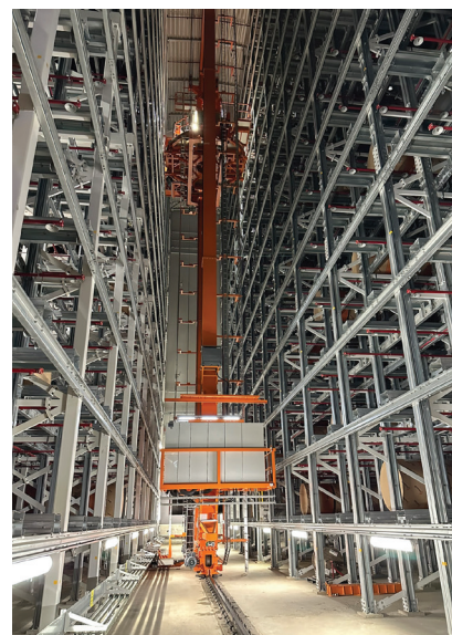
Figure 4 & 5: The deep-channel high-bay warehouse, with its high storage density, enabled Mondi Štětí to locate an automated storing and sorting buffer directly after the production line, despite the confined mill layout.
