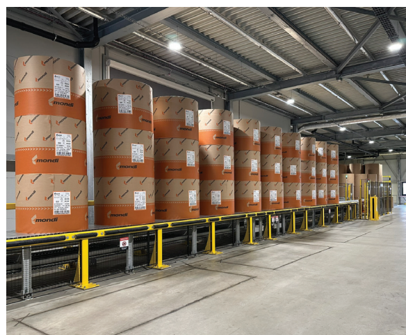
Figure 6 & 7: Up-ended roll stacks sorted on warehouse conveyor right after ARW for one touch "pick – turn - load" shipping process.
