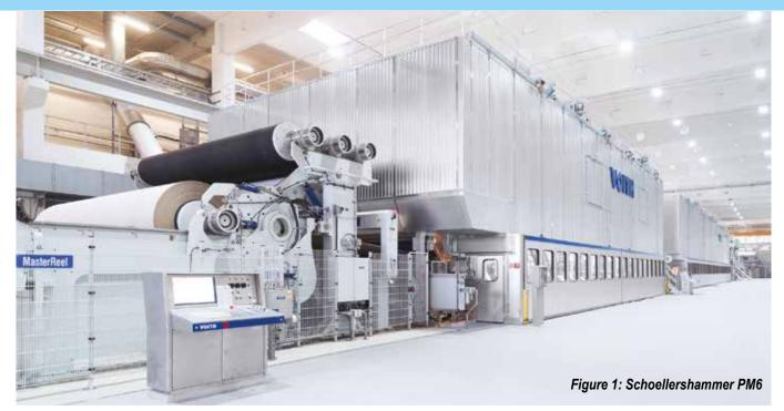
The impetus for the new machine goes back several years. At that time, Schoellershammer wanted to expand its range of packaging materials. In order to be able to produce efficiently here, the company decided to invest in another paper machine, the PM 6. It was to produce packaging papers in the basis weight range of 80 to 120 g/m2 to complement the PM 5. The goal was to achieve an annual production capacity of 535,000 tons of packaging paper with both machines.
