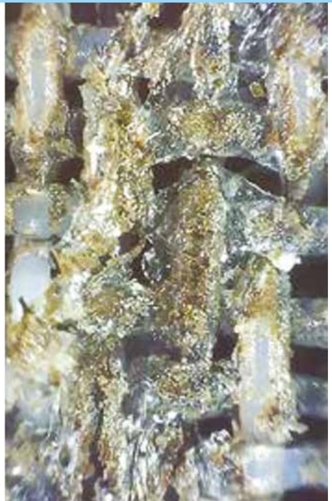
Figure 1: Typical "stickies" on a Forming Fabric.
