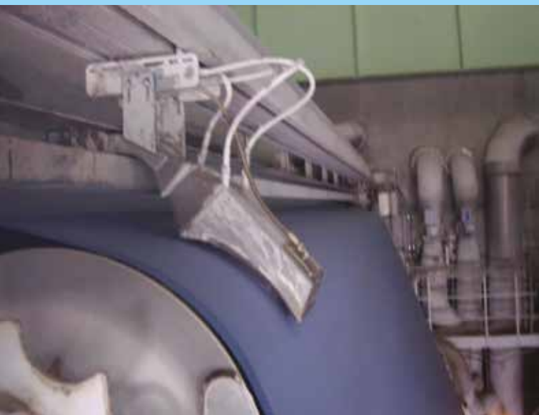
Figure 2: ProJet's ProCleaner in operation on a Top Former.
