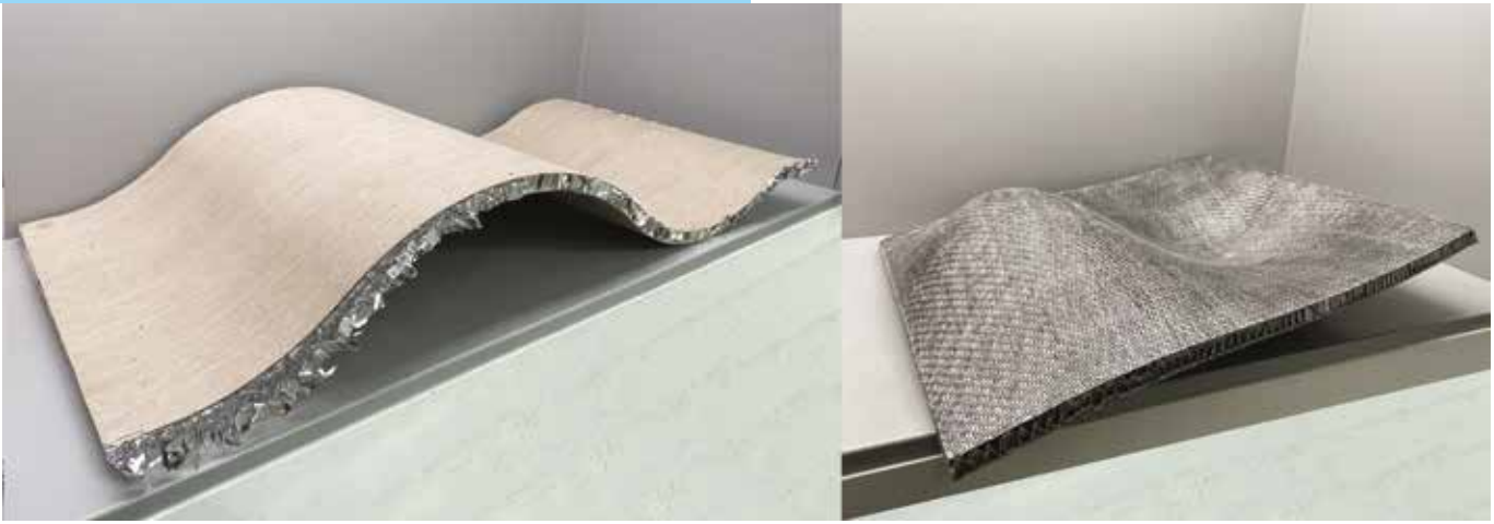
Figure 2: Single and double curved honeycomb moulded part.
