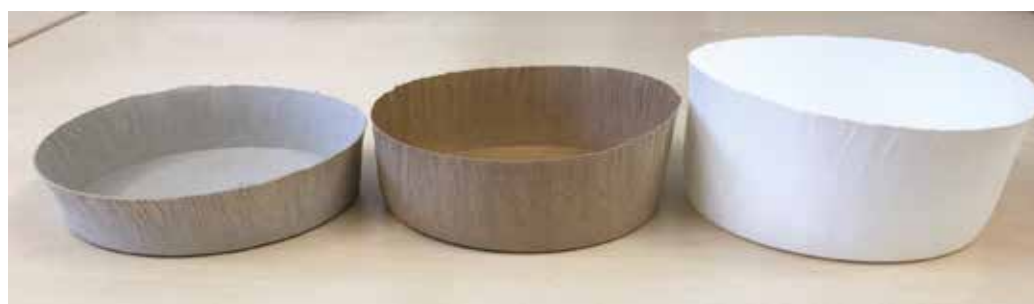
Figure 7: Different results of deep drawing in terms of the degree of deformation and number of folds due to the use of different materials.
