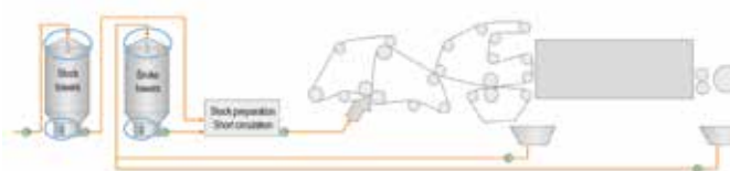
Figure 6: Sulzer TES, SALOMIX™ agitators and process pumps in paper mills.
