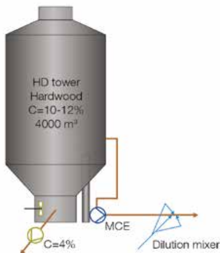
Figure 14: MC parallel pumping process application.
