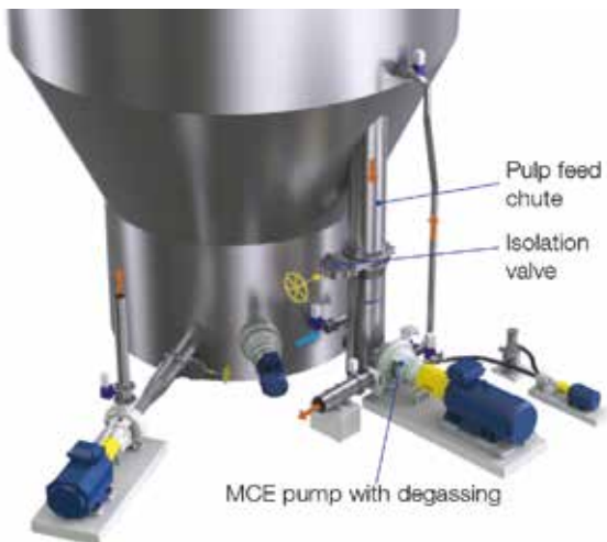
Figure 13: MC parallel pumping system arrangement.
