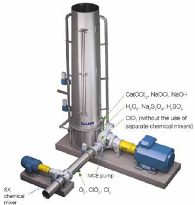
Figure 21: Chemical injection points in MC pumping and mixing system.
