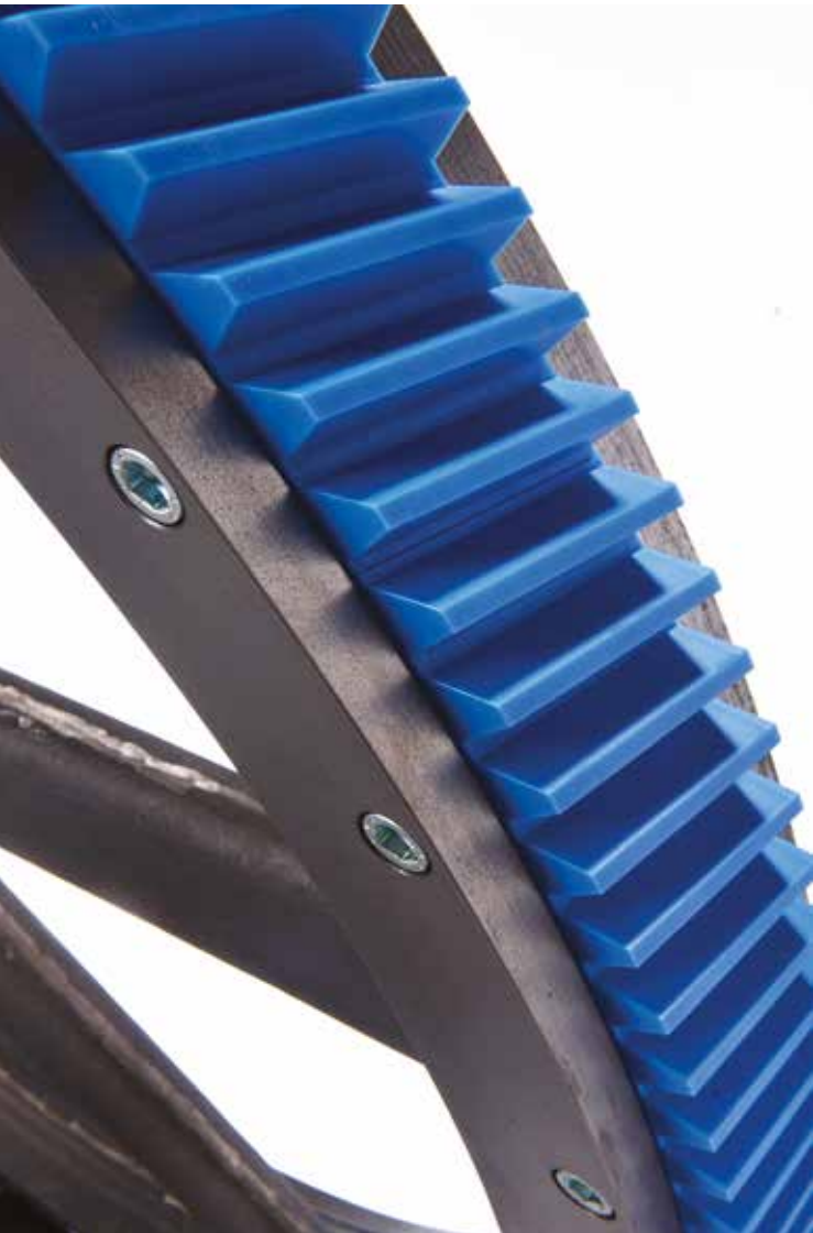
Figure 8: Gear wheel segments in Nylatec360 mounted on metal rim.
