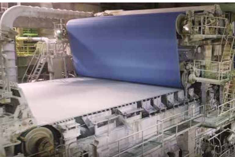
Figure 1: Forming section of a paper machine.
