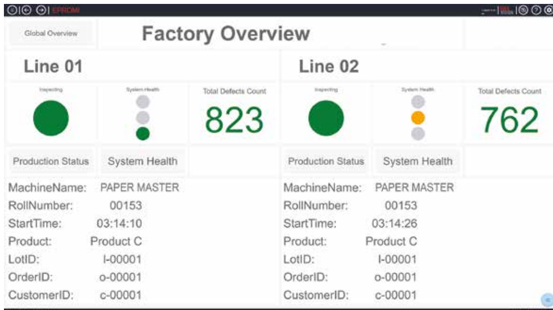
Figure 3: Connecting Information (quality and process) from different lines in the mill-wide system
