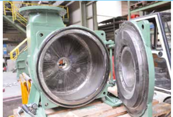
Figure 2: Highly wear-resistant regenerated housing.
