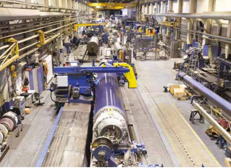
Figure 6: Roll-Grinding (in front) – Perfect results due to 3D-Steering with 4 Point measurement system.
