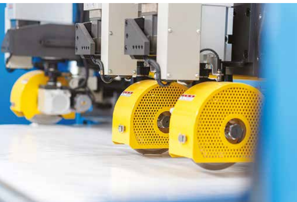
Figure 7: Slitting section on the sheeter.
