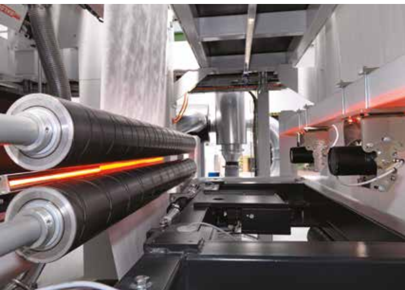
Figure 6: Automatic Edge guiding system.
