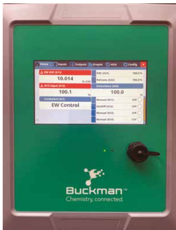
Figure 4: Controller for closed loop control of defoamer dosing.
