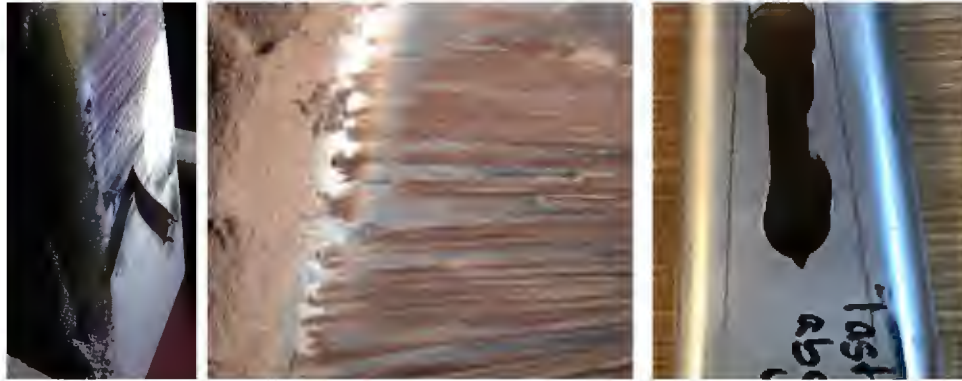
Fig. 6+7 Dryer fabric deposits at the guide palm
