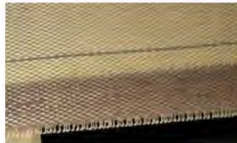
Fig. 10 Migrated dryer fabric MD yarns
