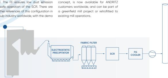
The innovative Lo-NOx recovery boiler concept combines various well-proven ANDRITZ technology solutions to achieve minimum dust and NOx emissions from the boile
