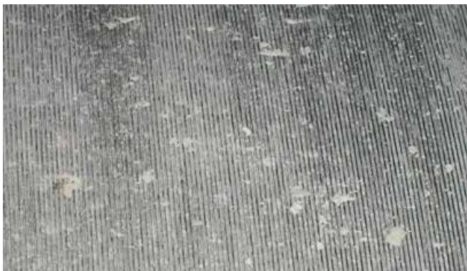
Grooved roll surface before RS AirBlade installation.
