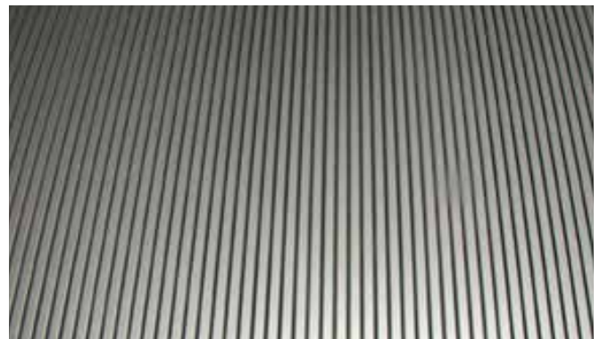
Grooved roll surface 2,5 years after RS AirBlade installation. Grooves are totally clean.
