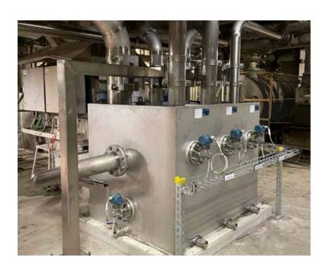
The EcoFlow Dewatering Measurement is designed to optimize dewatering and vacuum levels in the forming and press sections. EcoFlows also give you a unique window into the dewatering process.
