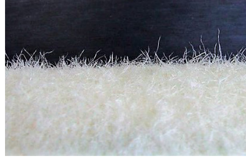
Fig. 7: Fiber stress at 30 bar significantly higher
