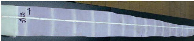
Fig. 12: Zonal felt wear visually identifiable in the used felt
