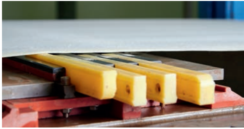
Fig. 15: Raised edge deckles on the Uhle box
