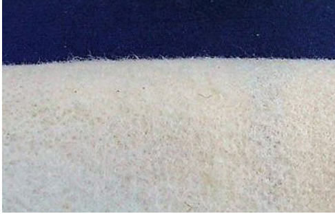
Fig. 6: Felt surface at 15 bar continuous operation
