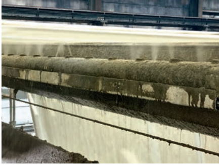
Fig. 9: Uneven water application
