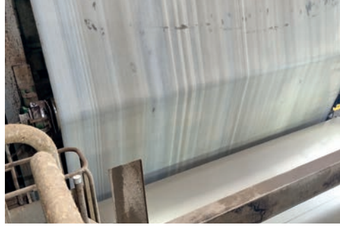
Fig. 10: Result: wet streaks in the felt
