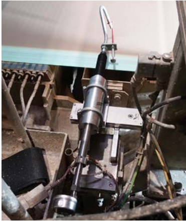
Modern edge trim nozzle system © PMS
