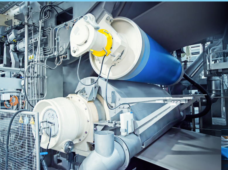
Figure 6: The combination of a 16 ft. PrimeDry Steel Yankee and the latest PrimePress XT Evo shoe press technology enables a high drying capacity and achieves remarkable cost savings and operational flexibility as well as improved product quality.
