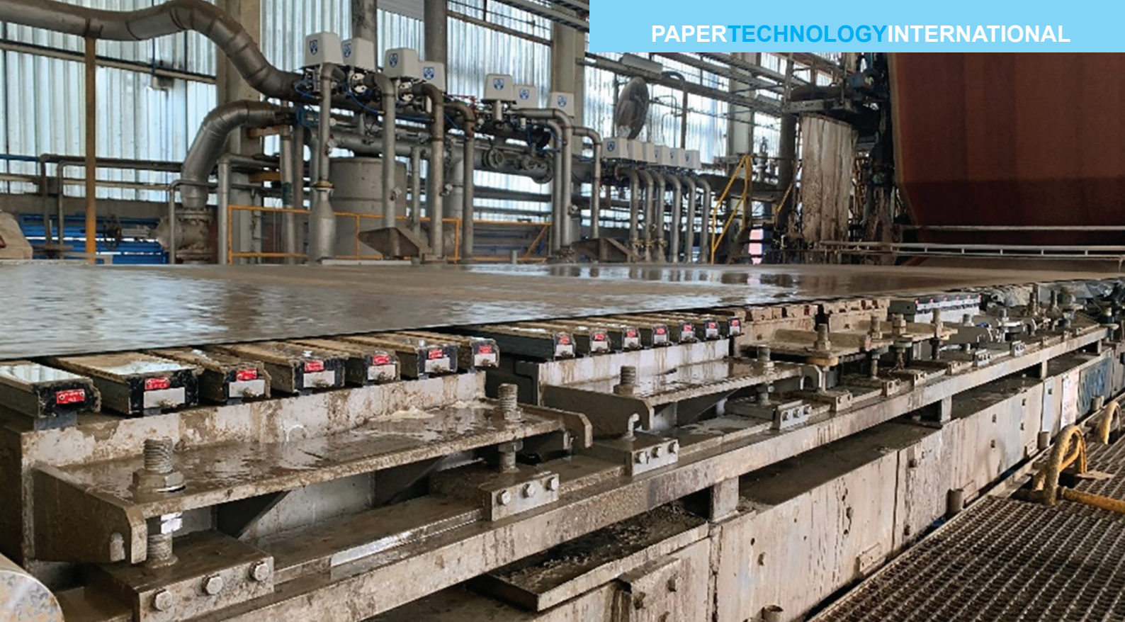
Figure 9: New wire table with SmartTable solution in Mexico.
