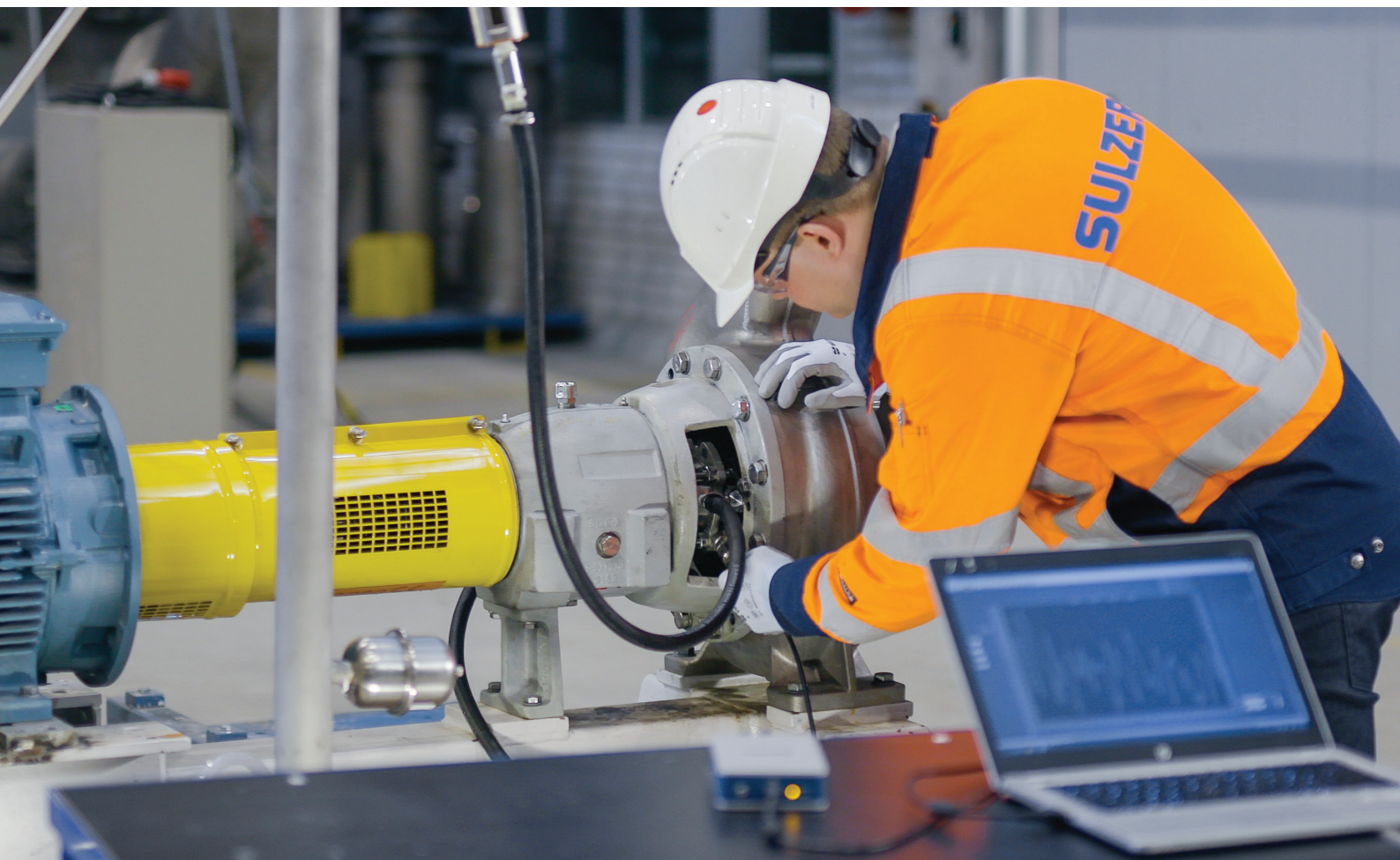
Figure 5: Mechanical seal testing at our full-scale research and development center.
