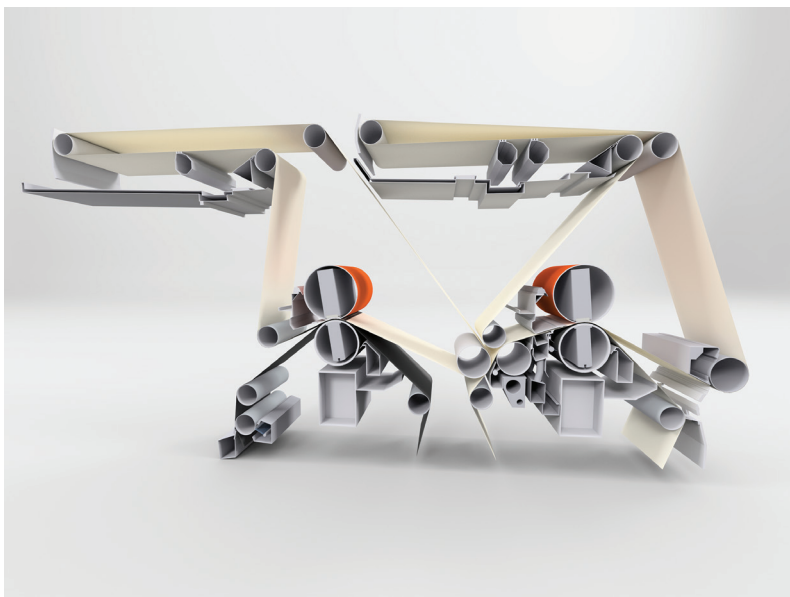
Figure 2: Voith's Tandem NipcoFlex press which combines two inline shoe presses is a press concept with a wide application window.
