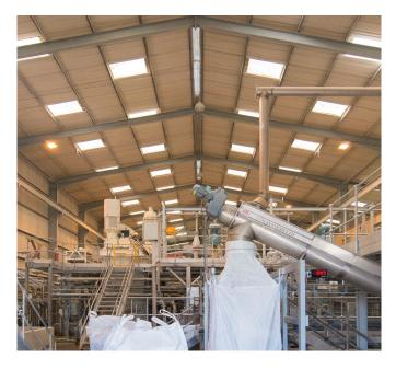
Figure 1: FiberLean MFC onsite scalable modules center around robust grinding technology. High-throughput continuous operation--Low maintenance costs and high uptime (>95% plant availability)--Chemical-free process--Highly-automated modular plant design with online monitoring.
