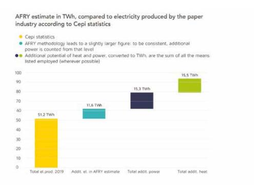
Figure 1: AFRY estimate in TWh, compared to electricity produced by the paper industry according to Cepi statistics
