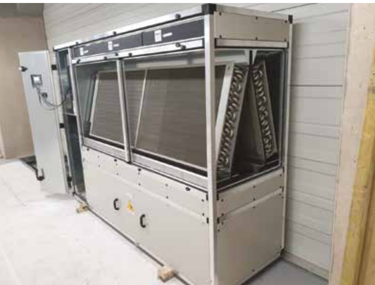
Figure 2: The Climate Cabinet: “Special Engineered Climate cabinet for the paper industry, with Siemens S7 control unit and A-shape coil to enable high natural cooling share for a year”.
