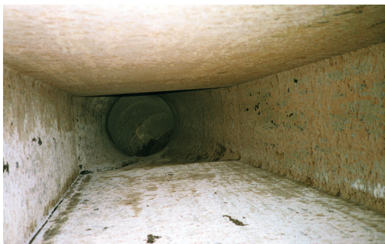
Figure 6: Head box with barium sulphate scale before cleaning.
