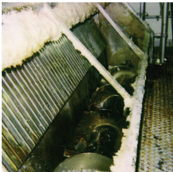
Figure 4: Conveyor screw covered with pitch- and talcum deposits.
