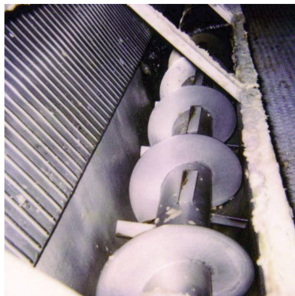
Figure 5: The same conveyor screw treated with pitch control agent.
