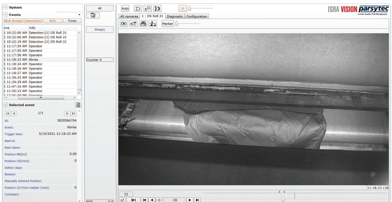
Figure 1b: With no actions taken, the web break has ultimately developed.
