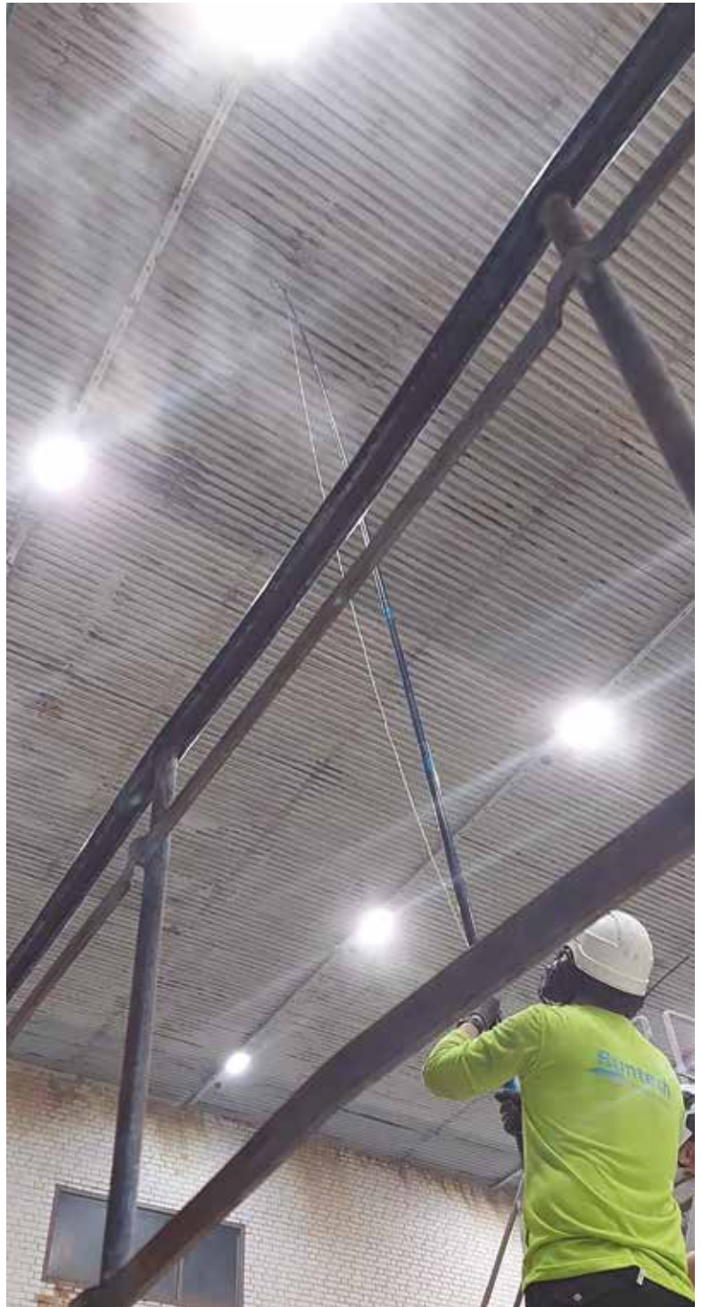
Figure 6: During machine hall ventilation audit air humidity is measured in the paper machine hall.
