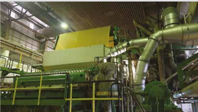
Figure 2 and 3: The machine hall before and after forming section and wet end ventilation at Kartonsan BM2.
