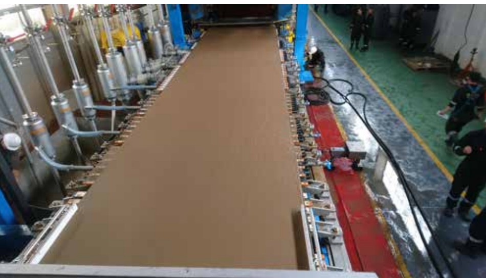
Figure 3: Fourdrinier machine functioning.
