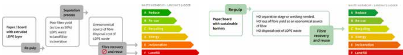
Figure 2 & 3: Circularity is created by making the fibre more economical to recover through existing recycling streams.
