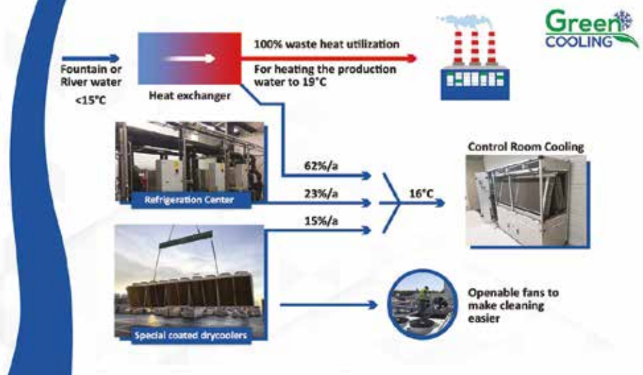
Figure 4: Original natural cooling concept diagram for Schoellershammer.
