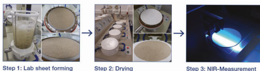
Figure 2: Procedure to measure stickies according to DIN SPEC 6745
