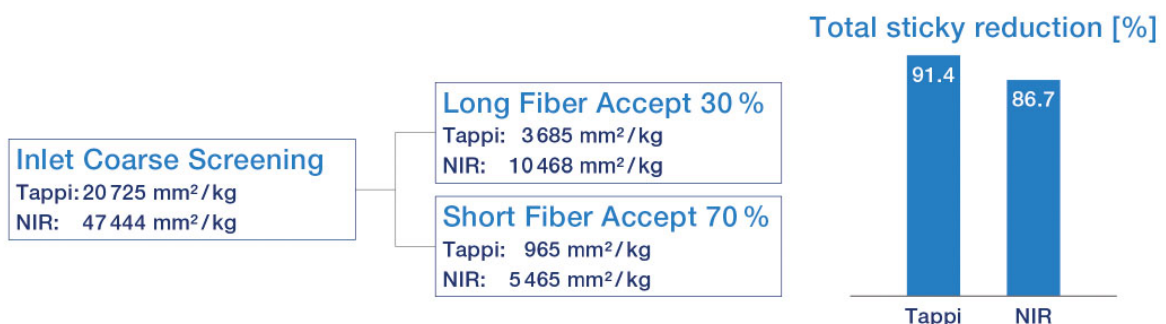
Figure 4: Sticky reduction for same process technology due to different measuring techniques – example for OCC samples
